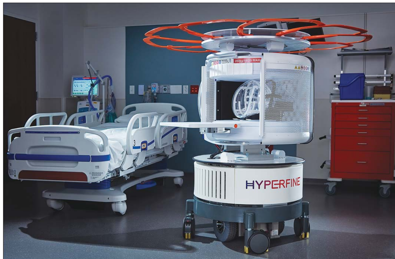
The Hyperfine Swoop MRI can be wheeled to the bedside and plugged into a power outlet on the wall. In minutes, it can determine if a patient has suffered a stroke.
